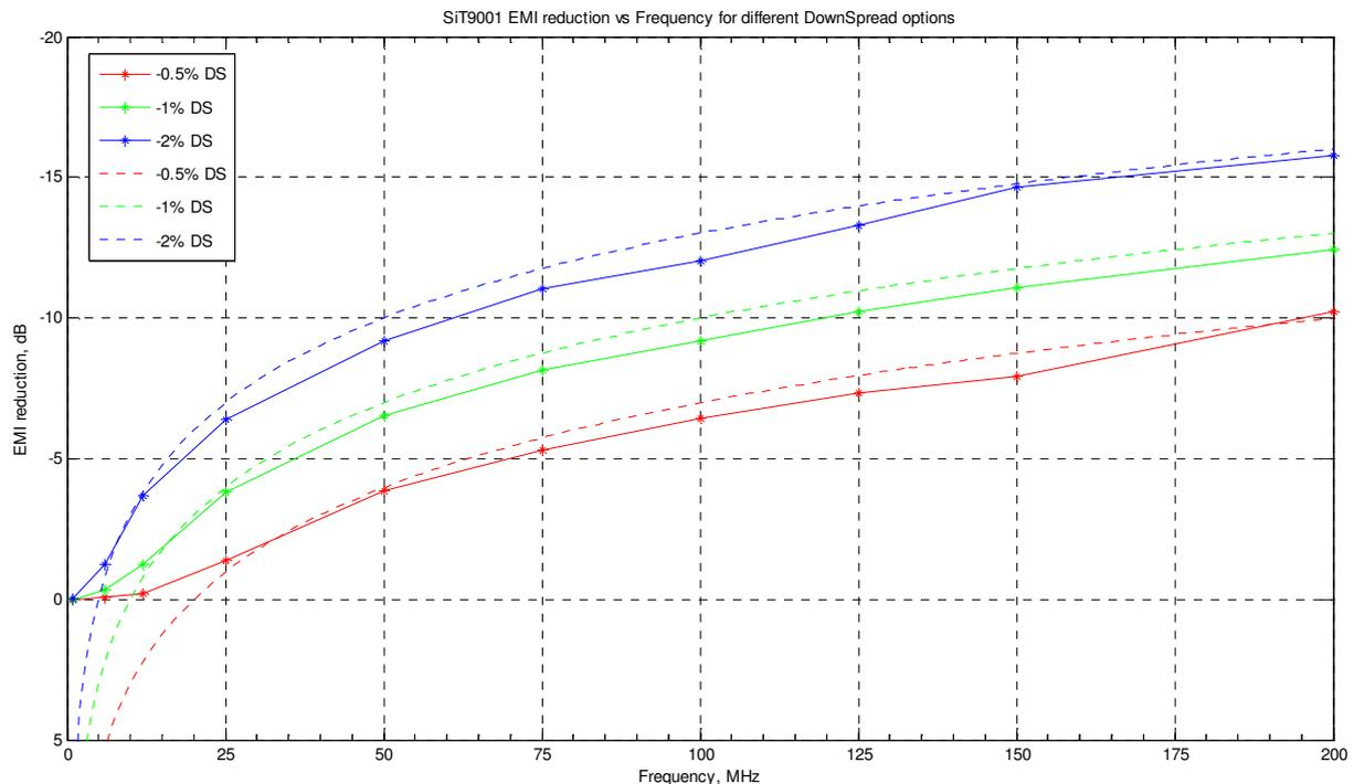
Figure 4. Calculated EMI Reductions vs Measured Values
