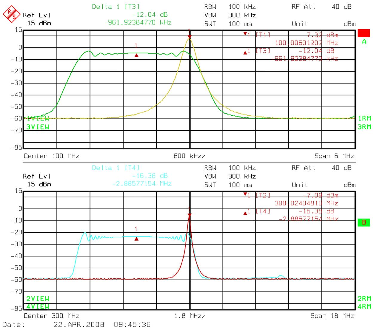
Figure 5. spectrum plots of a 100 MHz SiT9001 at 100 MHz and 300 MHz
