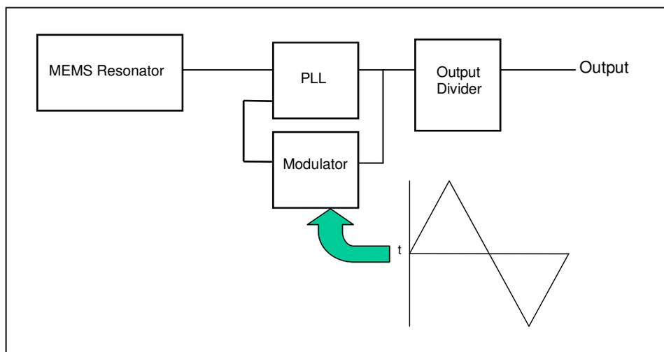
**Figure 1. Modulating the PLL with a Triangular Wave**
