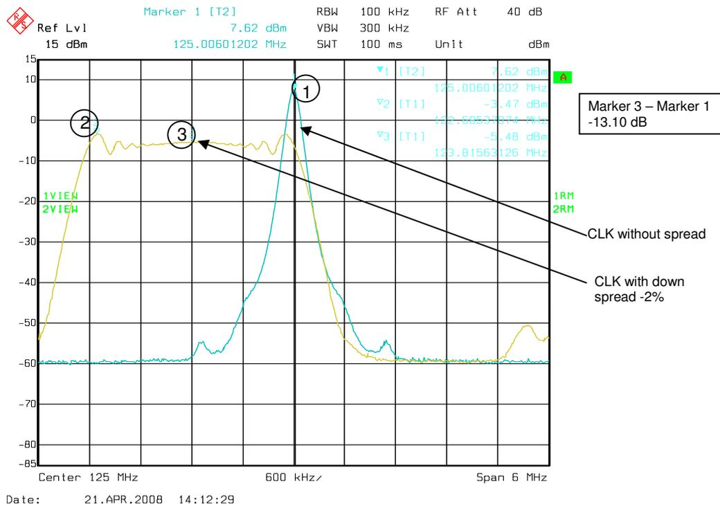
Figure 3. Noise Reduction Benefits of a Spread Spectrum Clock
