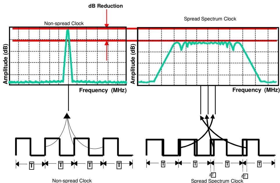
**Figure 2. Spectrum plots of a non-spreading clock and a spread spectrum clock as measured by a spectrum analyzer with a 100 KHz resolution bandwidth**
